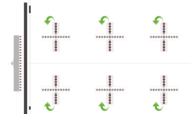
NDB301排钻示意图 Drills layout of NDB301
