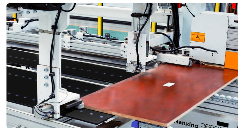
柔性辅助送料装置 (选配) Flexible side alignment device (Option)
